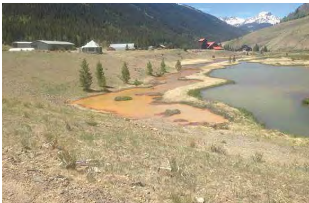
Figure 17. Effluent from buried mine tailings discharged acidic and metal-laced water into surface water. (Photo courtesy of Jon Kaminsky, Bureau of Land Management.)
