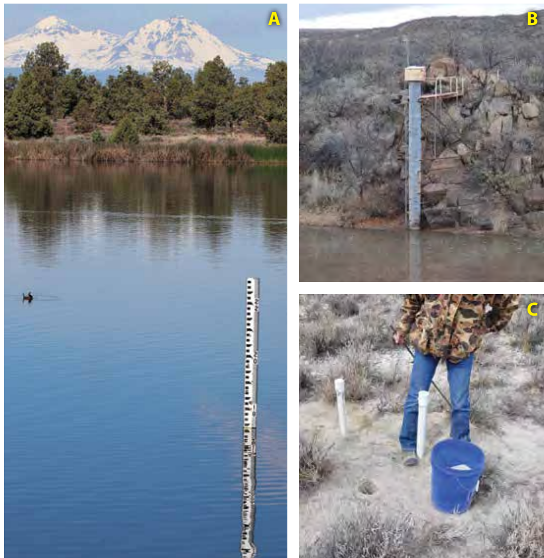
Figure 8. Staff gage (A) provides an inexpensive way to document changes in water stage. Stilling wells (B) and piezometers (C) also provide records of surface and groundwater stages. Many gages are outfitted with electronic recording devices to provide real-time, seasonal, and annual records of water-level fluctuations.
